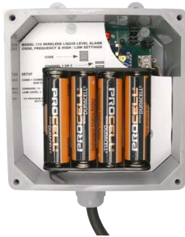
FIG 4 Outdoor Transmitter Batteries Installed
