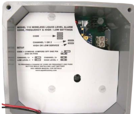
FIG 3 Outdoor Transmitter Enclosure Interior Close-up
