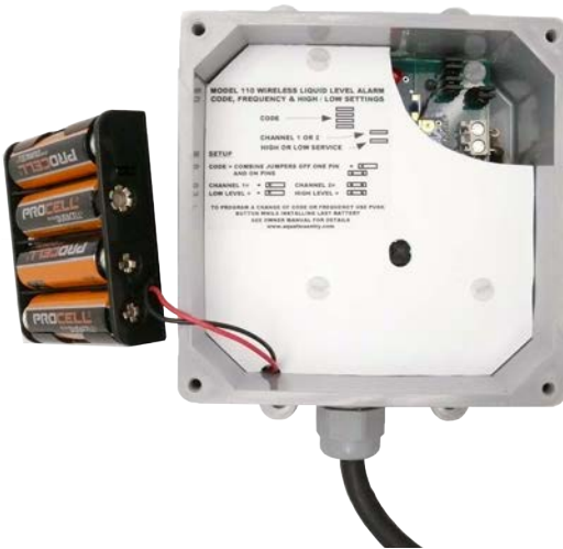
FIG 2 Outdoor Transmitter Enclosure Interior
